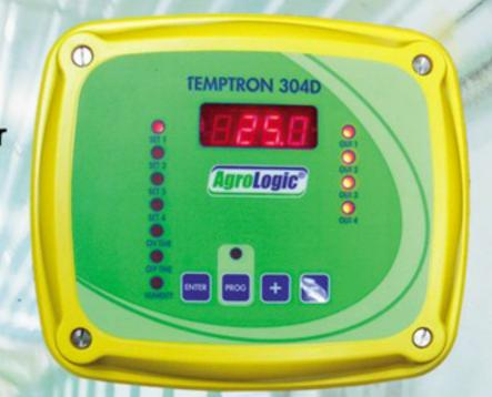
A humidity sensor can be connected to the Temptron
